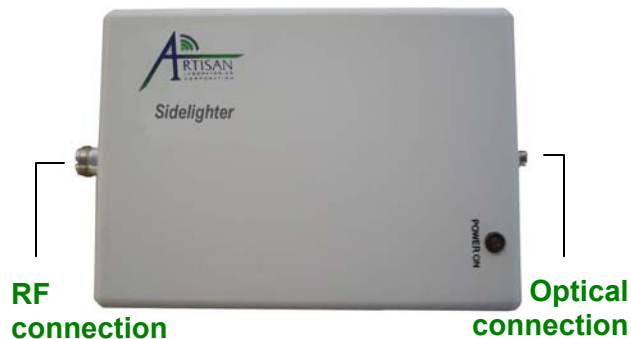
Figure 1. The Sidelighter is connected to popular microwave analyzers to measure distance to fault in fiber optic cables. Dead-zone free failures in fiber optic cables can be obtain with <10 cm resolution.
